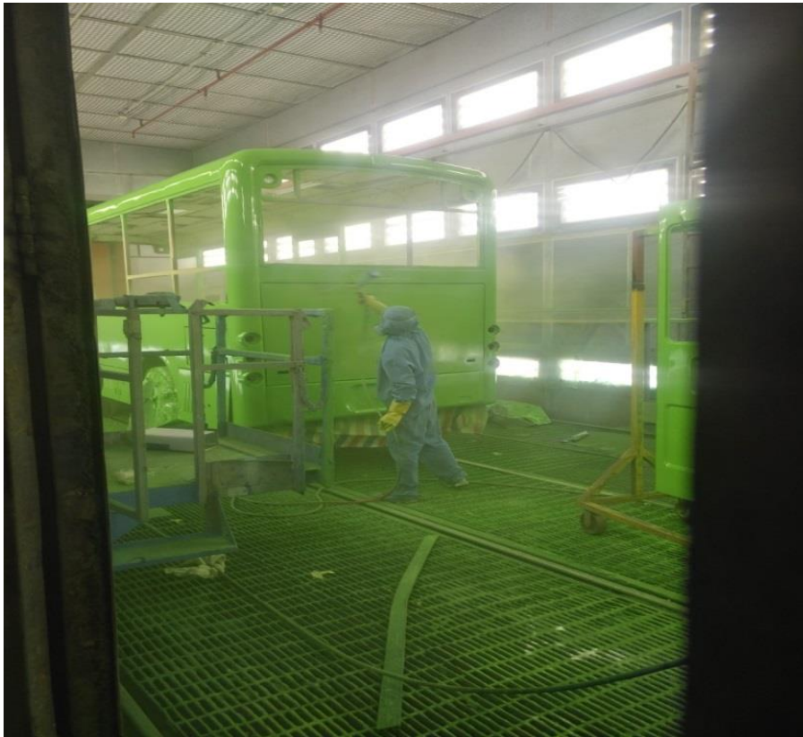
Antkote® 2035 used for topcoat of bus
